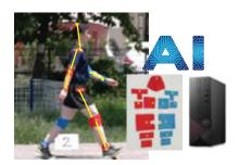
By combining AI-Based posture estimation with image recognition of specialized markers attached to the body, We have improved processing speed without compromising digitizing accuracy.
